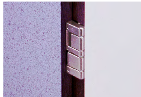
OBJECT HINGE (FA. PRAMETA) FOR COMPACT DOORS PANELS, DOOR THICKNESS 10 -13 MM. SINGLE AXIS PIVOT POINT.
